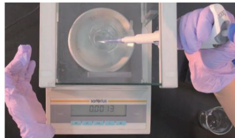
6. Repeat 3,4,5 in order to make adjustments and lock it when the setting has reached the target volume.
