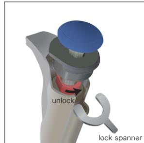
4. Adjust the volume by revolving the push button referring to the notch at the back of the button and lock it again.
